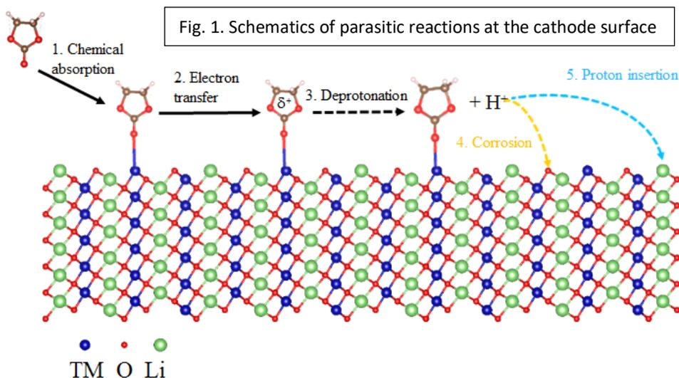
intermediate phase of cathode and the electrolyte, generating locally concentrated protons at the surface of the cathode materials. Figure 1 shows a generic mechanism of parasitic reactions occurring at the interface of cathode materials. Additional help from advanced characterization tools, such as synchrotron probes, will also be discussed.
